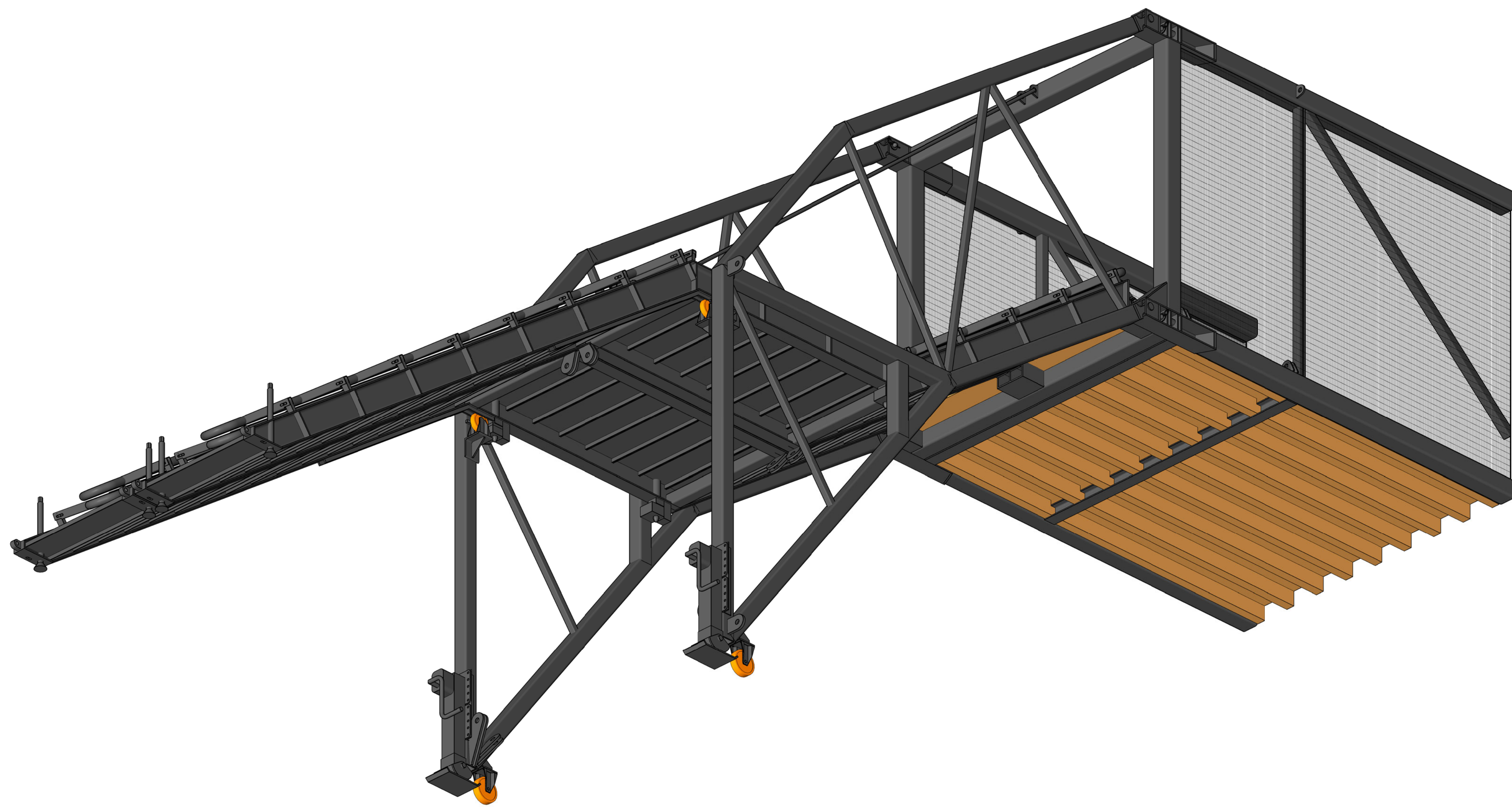
1 Isometric view of connection of stairs with legs underneath plateau scale
